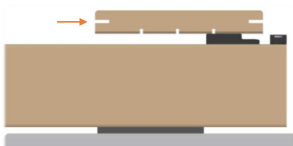
Figure 3: Fit the board on the substructure and press the lips into the holders.
